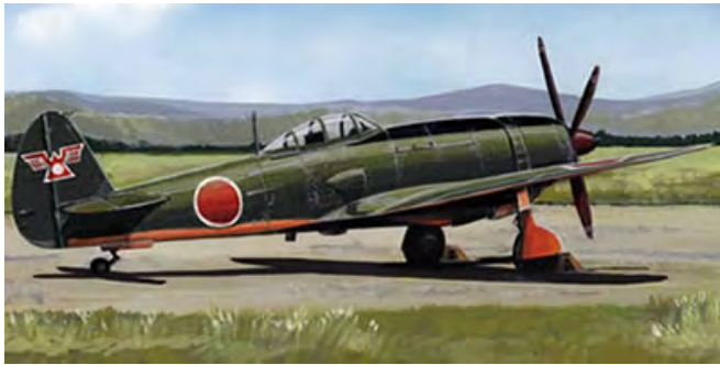
The Ki94 was powered by an 18-cylinder radial engine driving a 6-bladed constant speed propeller
