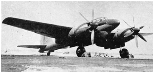
The engines fitted to the Ki.93 were a pair of 1,970 hp Mitsubishi Ha.214 18-cylinder radial engines.
